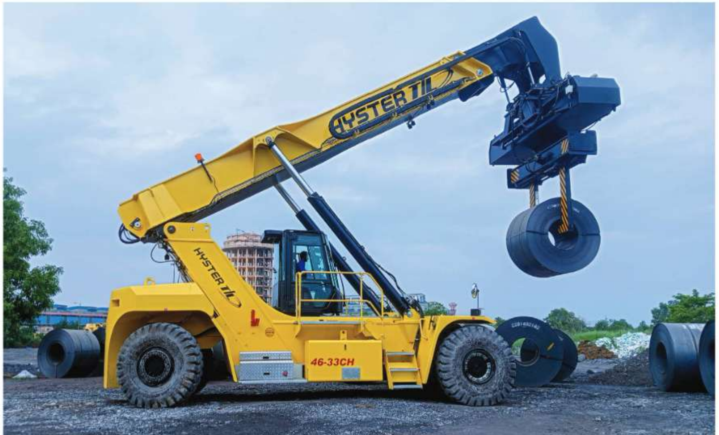
▲ The Rough Terrain Empty Container ReachStacker is tailored for India's often unpaved and challenging terrains.
