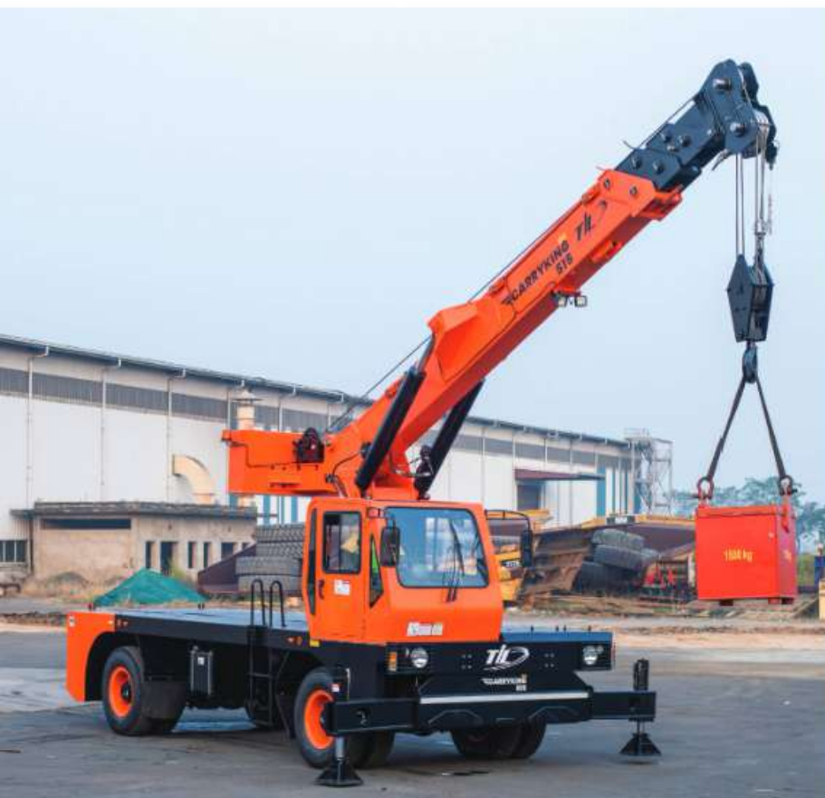
▲ The CarryKing 515 replaces three conventional machines by combining lifting, loading, and transportation capabilities on a single flat deck.
