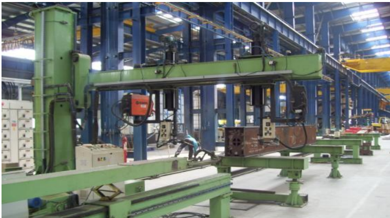
External Internal Auto weld m/c
