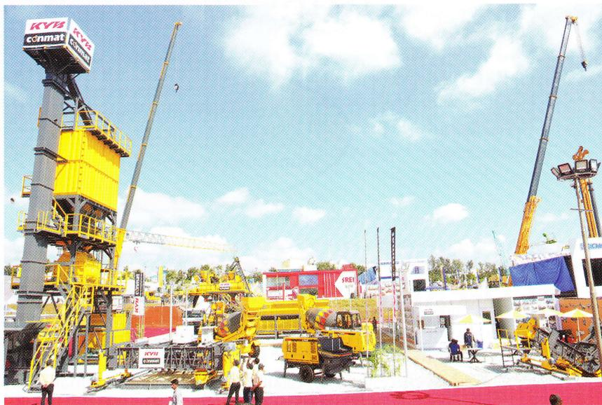
New product on display was the compact batching plant with sidewall conveyors, which can achieve a steep angle up to 50 degrees as compared to the 17-18 degree by conventional conveyors. It gives a 10% better output as compared to other batching plants. With this new sidewall conveyor, the batching time is reduced to 50 seconds since the conveyor is very short and runs at a very high speed. The plant gives higher productivity, lower fuel consumption, and enables easy application in constrained
