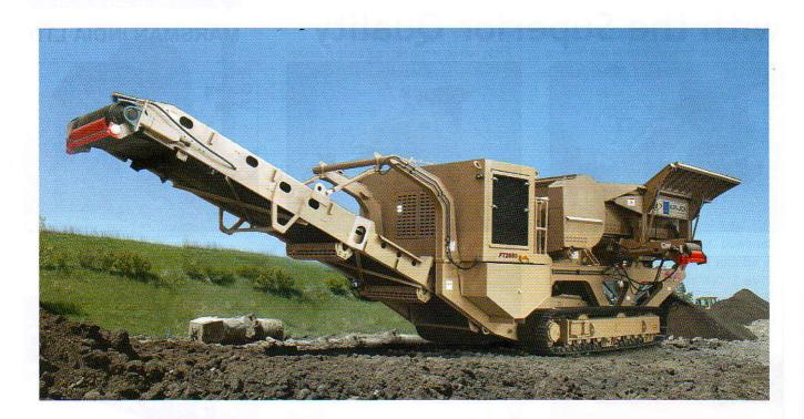
TIL Limited, has been carrying out value added improvisations in its 300 tph track mounted and 200 & 300 tph portable plants for making them adaptable to Indian operating conditions. The plants are manufactured under technical collaboration of Astec of US at its new plant in Kharagpur near Kolkata.
